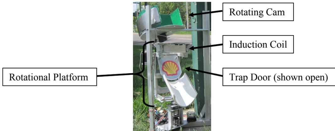
**Figure 1. Physical Components of Recyclable Material Sorter**
